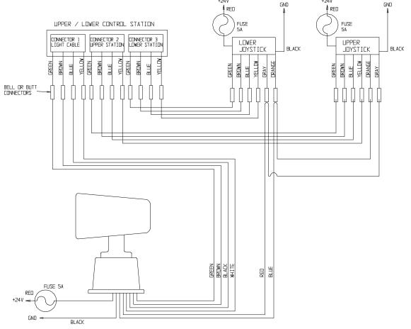
2. Connect the wires from the light, existing control panel, and dual station control and selector station as shown:
