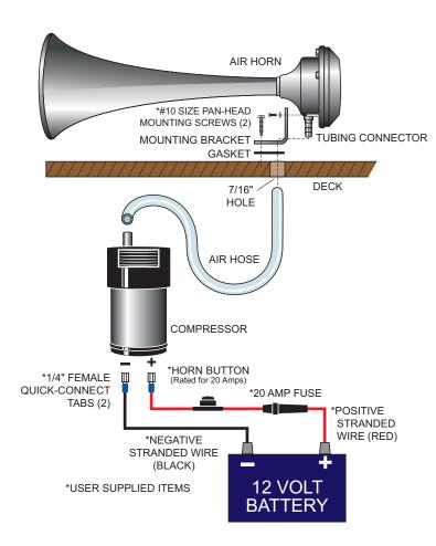
fitting and pressing it up about 1/2". Reinstall the horn to the mounting bracket with the two phillips-head screws. Use a small amount of silicone sealant to seal any gaps between the air hose and opening hole to prevent water from leaking inside. Make sure not to squeeze the air hose as this will impede the air flow.
