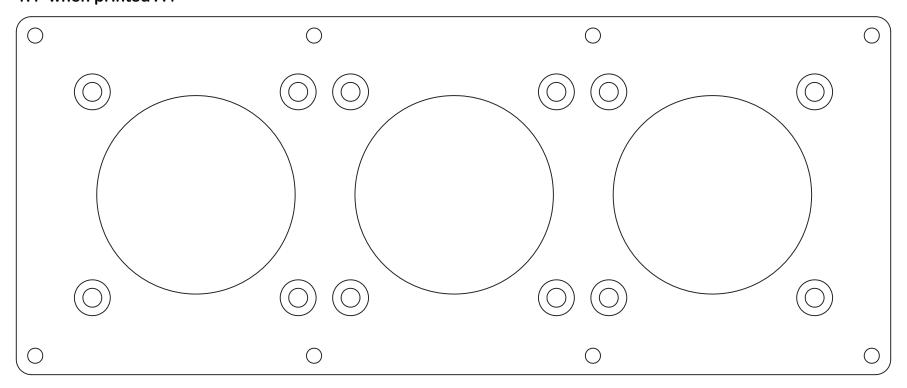
BSP-3L 380 x 170mm to suit 720 battery switches 1:1 when printed A3
