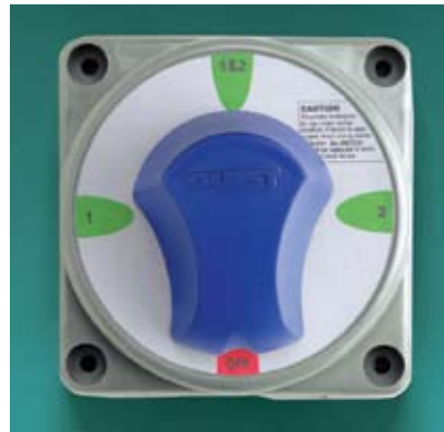
Battery Selector Switch Continuous Amps: 360 Momentary Amps: 600
