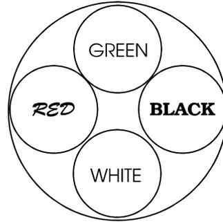
2. Insert the black and green wires into the "Y" and "G" terminals, and tighten the two terminal screws. **Note:** The drawing shows the plug. The "Y" terminal is on the other side on the connector.
