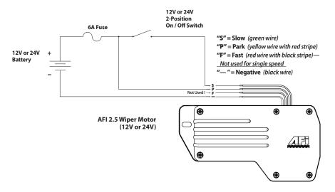
**Caution:** When wiring this two-speed motor as a single-speed you must use the slow speed as shown in the wiring diagram above and not the fast speed. Using the fast speed will ultimately cause the motor to over-heat and short out.
