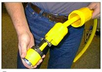
**5** Lubricate mouth of boot and rear shoulder of device with soap solution and pull into place.
