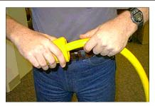
**2** Push cord through the inverted end about 18". A tug in the opposite direction returns boot to its original shape.
