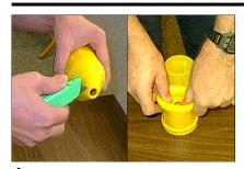
1 Cut boot at first line, if cord is greater than 5/8". Invert tapered end of the boot and apply soap solution.
