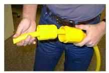
**3** Push cord through the plug/connector housing.
